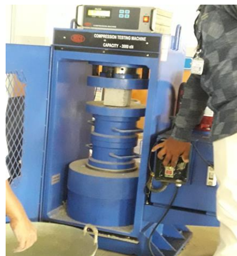
Fig. 3. Specimen testing in Compression Testing Machine
