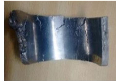
Fig. 2. The specimen showing the Aluminum copper metal matrix composite before rolling
