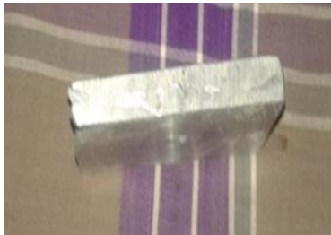
Fig. 1. The finger mold made by the stir casting method
