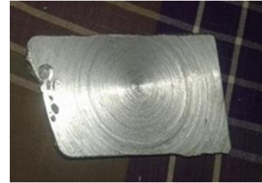
Fig. 3. The rolled specimen showing the convex shape after rolling.
