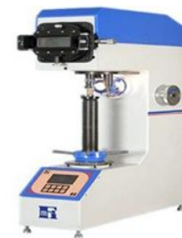
Fig. 4. The Vickers hardness-testing machine which is used for testing the hardness of the derived samples
