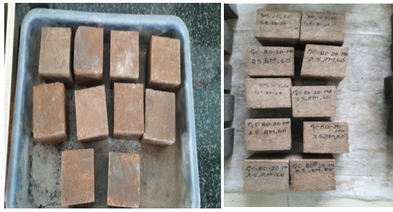
g) After demould Fig. 5. Steps to prepare GPM cubes
