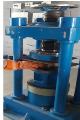
a) Placing of cubes in CTM
